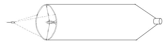
Figure 2. The bongo-net used for collecting fish larvae
